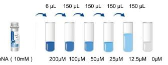
3) Take 100 µL of different concentrations standard solutions to the cuvettes or wells of microplate and detect the OD value at 405 nm (In order to ensure the accuracy of experimental results, it is recommended that all samples and
